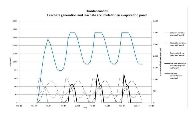
Figure 8 Leachate generation and leachate accumulation in evaporation pond at Hrazdan landfill (Leachate pond 4,000 m² and 3,000 m³
